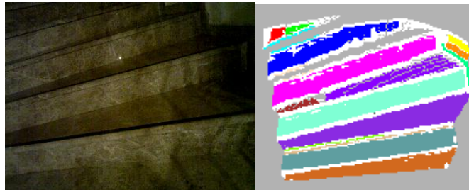
Figure 9. One image of spiral stairs and its point cloud segmentation result
